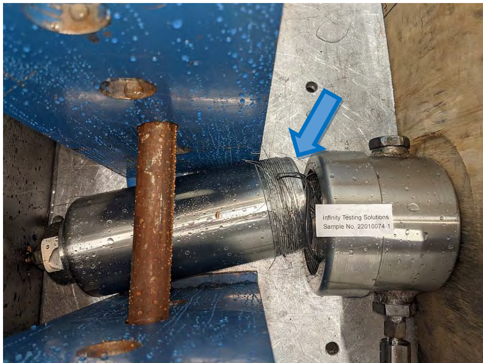
Figure 2: Sample 22010074-1 burst, maximum pressure achieved 21,943 psig
